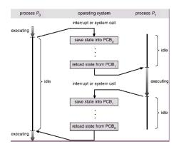
Figure 6: Process states of a interrupt request
