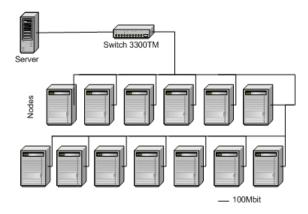
Figure 1: Test setup openMosix cluster
