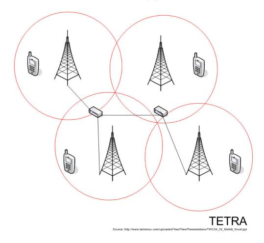
Figure 4.1: Example of a TETRA network setup. The network is based on masts – connected with cables – and mobile communication units.
