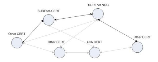
Figure 5.2: Communication in an Emergency Network, simplified. Black arrows represent real communication, grey arrows represent possibilities to communicate
