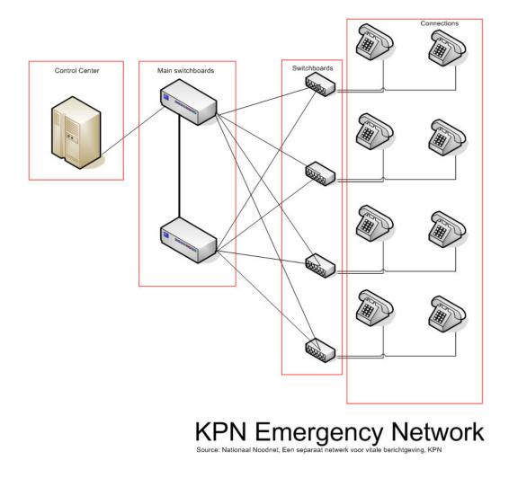
Figure 4.2: Infrastructure of the KPN Emergency Network, a simplified version.
