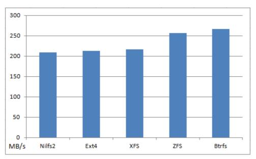
Figure 1: Sequential read performance of file systems on a single SSD.
