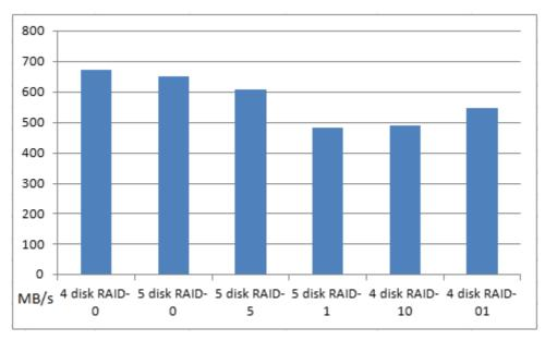
Figure 3: Performance of different software RAID levels with Btrfs on SSDs.
