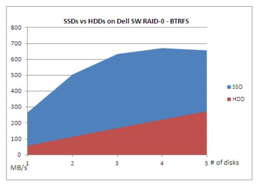
Figure 2: Performance of Btrfs on SSDs and HDDs on software RAID-0.
