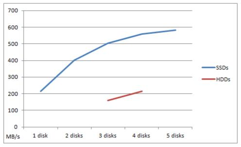
Figure 7: XFS file system software RAID-0 scaling over SSDs and HDDs.
