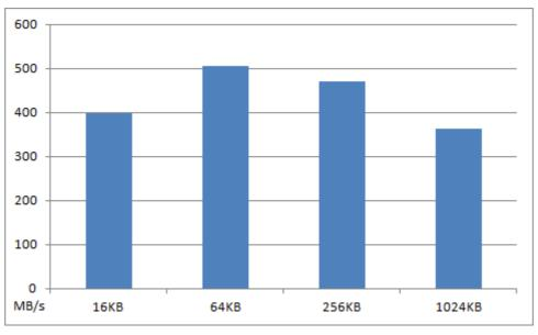
Figure 4: Hardware RAID-0 stripe size on 5 SSD array with Btrfs.
