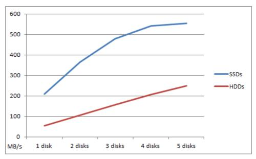
Figure 6: Nilfs2 file system software RAID-0 scaling over SSDs and HDDs.
