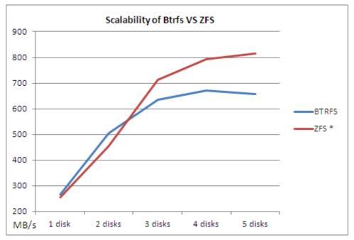
Figure 8: Btrfs and ZFS scaling on SSDs.
