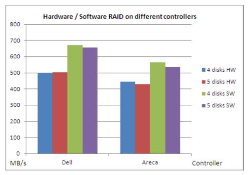
Figure 10: Comparison of software and hardware RAID-0 on the Dell Perc 6/i and Areca ARC 1680 controllers performed with Btrfs.
