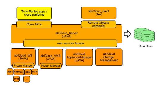
Figure 8: Platform architecture of AbiCloud.[11]
