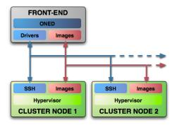
Figure 6: Topology of the architecture of OpenNebula. [28]
