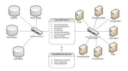
Figure 9: Topology of the architecture of OpenQRM.[37]
