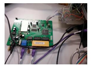
Figure: A DLC5 Cable is used to connect a TP-Link 1043ND with a standard PC.
