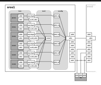
Figure : Interconnections of (virtual) interfaces on sros1
