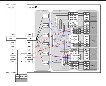
Figure : Interconnections of (virtual) interfaces on sros2
