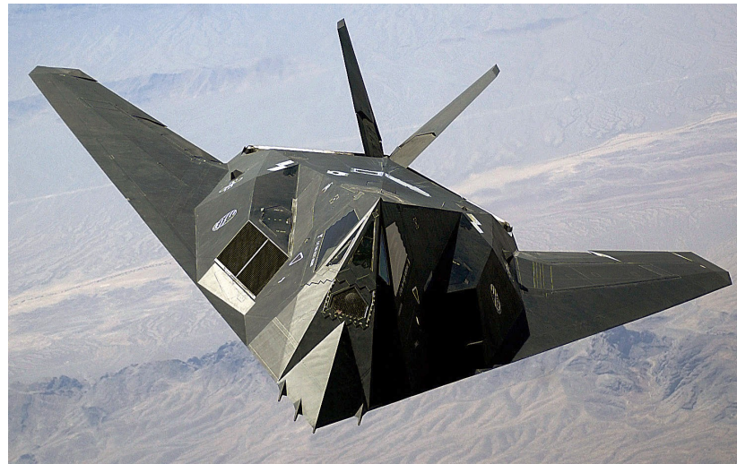
Figure 5: The US F117 is a 13m wide airplane, but under the radar it appears to have the same size as a bird.
