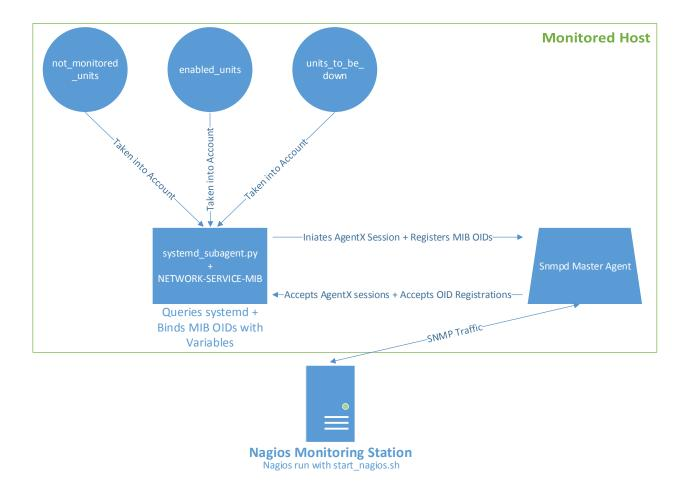
Figure 1: The workflow of the proof of concept
