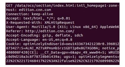
Figure 13: HTTP headers after processing by tcpflow
