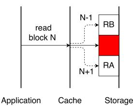
Figure 3: Read-ahead (RA) and read-behind (RB) comparison
