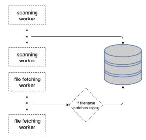
Figure 5: triage.py architecture overview
