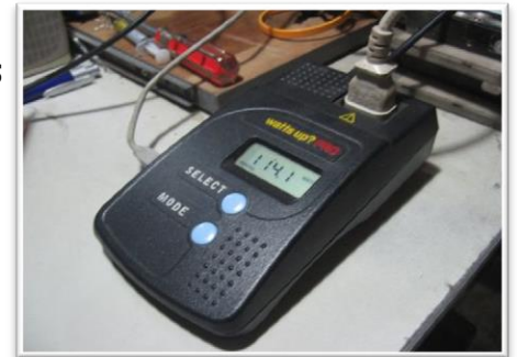
Figure 1: Power Measurement Device
