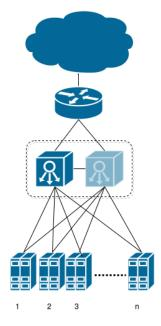
Figure 1: Load balancing with an active (dark blue)/passive(light blue) setup. This setup scales up to n hosts depending on the capacity of the Load Balancers
