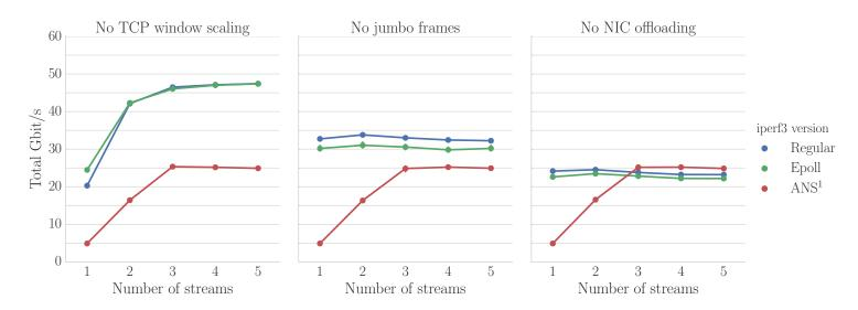
Figure 8: Performance comparison with the missing ANS performance features disabled separately for Linux
