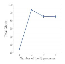
Figure 4: iperf3 test with multiple processes
