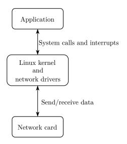
Figure 1: Regular networking on Linux
