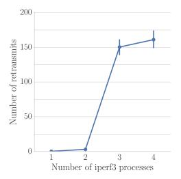
Figure 5: Number of retransmits for multiple iperf3 processes
