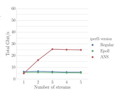
Figure 9: Performance comparison without all the features that are missing in ANS
