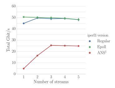
Figure 7: Performance comparison with multiple TCP streams and optimal settings
