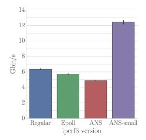
Figure 10: Performance comparison with a single TCP stream with performance features disabled that are missing from ANS
