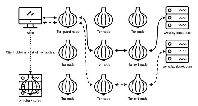
Figure 2.1: Step 1 (dotted): The client connects to the Tor directory servers to retrieve a list of Tor nodes. Step 2 (solid): The client connects through Tor to www.nytimes.com. Step 3 (dashed): The client connects through a different circuit to www.facebook.com.
