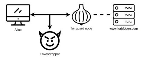
Figure 2.2: An attacker is eavesdropping on the communication between the client and the guard node and can infer based on the metadata of the TCP/IP stream which website the client is visiting.
