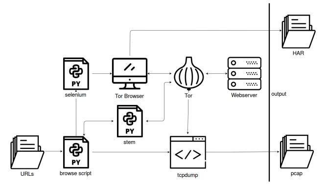
Figure 3.1: An overview of the setup used in the experiments.
