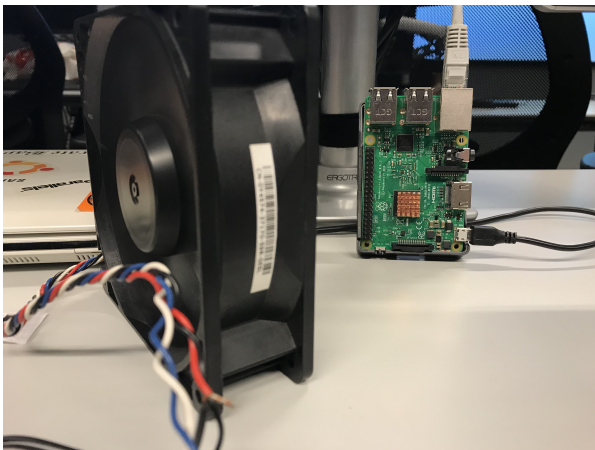
Figure 14: Raspberry Pi 3 extra cooling
