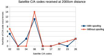
Fig. 16. Detected C/A codes at a transmission power of 10 dBm.
