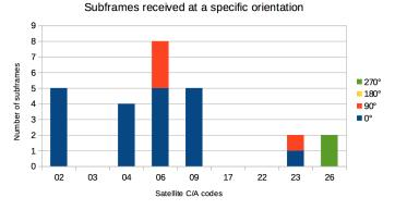
Fig. 19. Second test of Subframes acquired from one frame at specific orientations
