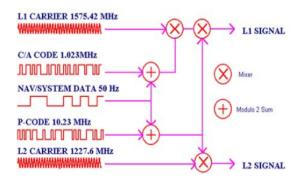
Fig. 2. Modulation of the L1 and L2 GPS signal[32]
