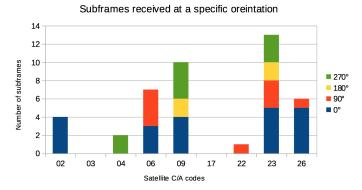
Fig. 18. First test of Subframes acquired from one frame at specific orientations
