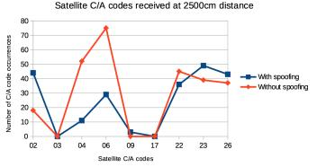
Fig. 15. Detected C/A codes at a transmission power of 8 dBm.
