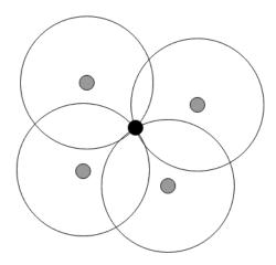
Fig. 1. Trilateration example with four satellites
