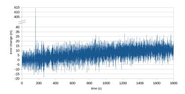
Fig. 21. Changes in the 3D error over time of run 2 with the monopole antenna
