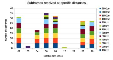
Fig. 13. Subframes acquired from one frame at a transmission power of 8 dBm.
