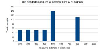
Fig. 12. Time required to acquire a GPS location with a transmission power of 10 dBm.
