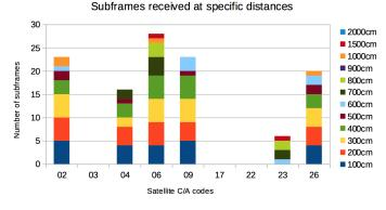
Fig. 14. Subframes acquired from one frame at a transmission power of 10 dBm.
