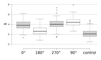
Fig. 17. Tukey box plot of power level per orientation in dB
