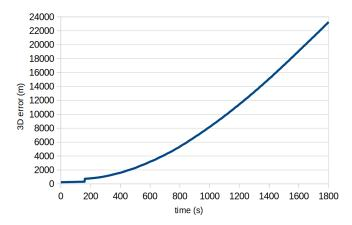
Fig. 20. Longitude, latitude and altitude error (3D) vs. time of run 2 with the monopole antenna
