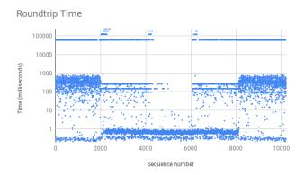
Figure 3: Roundtrip time during cache scaling events
