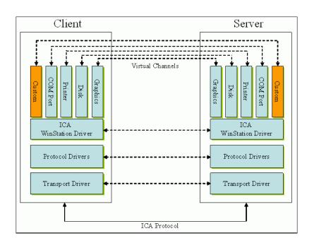
Figure 2: Image describing how virtual channels are managed using WinStation [9]
