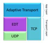
Figure 1: Adaptive transport contains Enlightened Data Transport and TCP [5]
