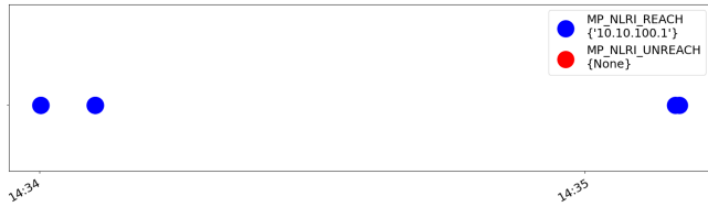
Fig. 5. Plot of incorrect received reachability information. The y-axis represents the type of advertisement, while the x-axis the time, with format HH:MM.
