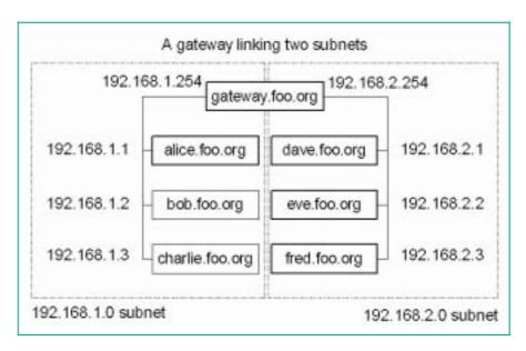
Figure 6 - A gateway linking two subnets.
